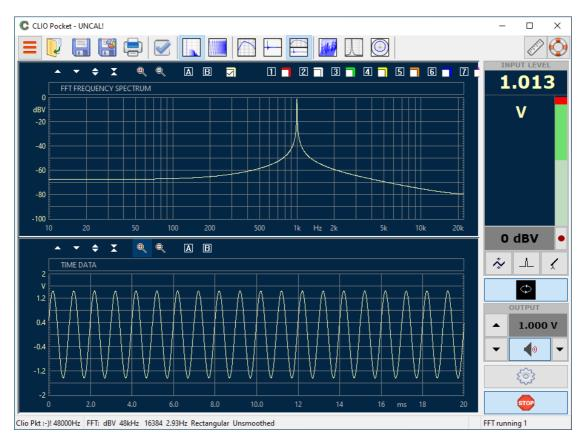
The result you should obtain is an FFT analysis of the 1kHz sinusoid and its time representation given by its waveform.
