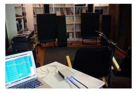
Unlike Log Chirp measurements, FFT and RTA are interactive; the user can chose either to generate a particular stimulus signal or simply analyze what is present at the mic input. When possible, when using a stimulus, it is advisable to use CLIO's internally generated signals because they lead to more precise and powerful analyses. Here we describe two examples exploiting both methods.
