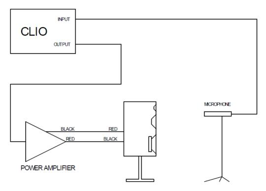
Note that the polarity of the cable from the amp to the loudspeaker is inverted. This
