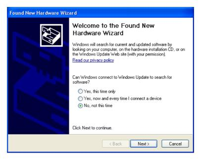
The wizard will direct you while installing the two drivers needed. You should *Install from a specific location* and point to the driver folder for XP on the CD (usually  $\$  Windows $\$ Driver $\$ P) and then answer **Continue Anyway** to the prompt about Windows Logo testing.
