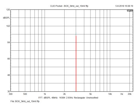
We then increment the driving level at 1 dB steps. As soon as the system starts to go over its linear range, a set of harmonic components of the input tone will appear at the output.
