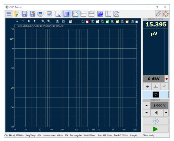
You can click on the marker  $\boxed{\mathbb{A}}$  button and inspect the amplitude of the measured signal: you should obtain a reading around 0dBV, this is the correct output level of the LogChirp signal with the generator output set to 1V.
