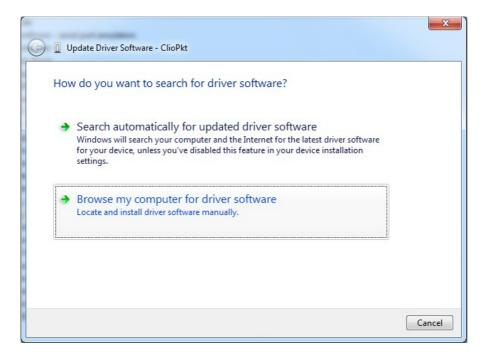
Browse your computer and point to the folder inside the installation SD card where the proper drivers are located (usually \Windows\Driver\Vista\_7\_8).
