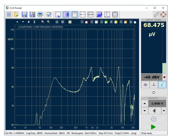
Repeat measuring and adjusting Input Gain until the maximum before overload. In the figure above we have it set at -40dBV (10mV) full scale which is the highest possible Input Gain. Depending on the speaker this might change. You can also safely increase or reduce the Output level to keep the response within 80 to 90 dBSPL. You should obtain a Pressure Frequency Response even if, for several reasons, **it is not the real one of the speaker**.
