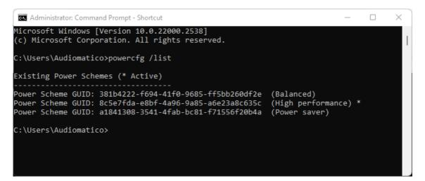
When using a notebook **never run on batteries**, always hook it to AC mains, as power saving schemes greatly reduce performances. As ultimate resource these are Recommended Advanced Power Settings, i.e. set 100% the Minimum processor state:
