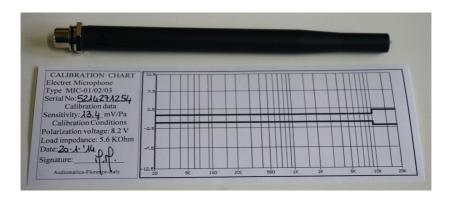
In the case of figure input 13.4 mV/Pa in the Pressure>Sensitivity edit box.
