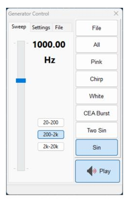
The three bands continuous sweeper that can be operated with the associated slider. The normal Coarse control (over the entire frequency band) can be changed (pressing Ctrl) to a Fine tuning of  $\pm 1\%$  centered around actual frequency.
