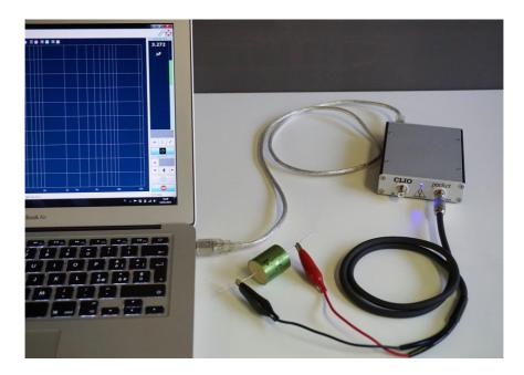
Click on the Units label within the Level Meter and select the correct measurement units for the component under test (Resistance, Capacitance, or Inductance). Then press the <a> arrow that starts all measurements and you should see a real time measurement.</a>
