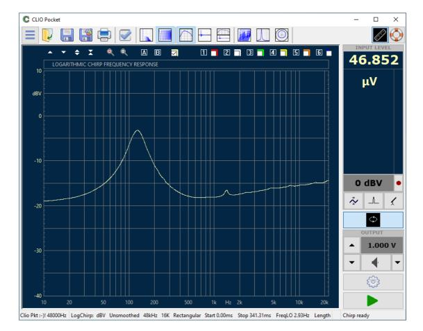
Actually this is not an Impedance Curve, but a Frequency Response showing the log scaled voltage division of CLIO's output impedance with the loudspeaker's input impedance. Open the LogChirp Settings <sup>(2)</sup> and change both Size to 65536 and Units to Ohm.
