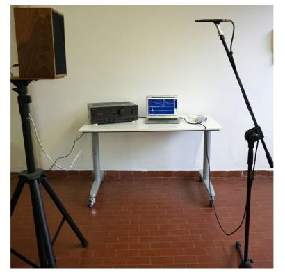
Up to now what was in the CLIO box was sufficient. To proceed now you have to connect your own audio power amplifier via an an RCA cable. The amplifier should possess a flat Frequency Response and a low output impedance. Check that the CLIO generator is turned OFF  $\P$  and that the amplifier is turned OFF. Connect CLIO's Output to the amplifier input and the amplifier's output to the speaker you are measuring. Refer both to the above picture and the schematic below
