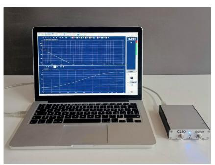
Upon a successful installation the front panel blue led should now light up, you may hear the internal relays clicking and the program should start smoothly and present the main desktop.
