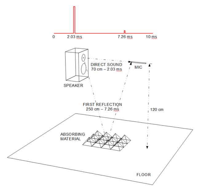
In the above figure you see the common practice of placing absorbing material to attenuate the first reflection. However be advised that, as long as this affects only high frequencies, it has the disadvantage of masking the exact arrival time by slowing the rise of the reflected impulse. Therefore, it is ideally better to delay the arrival time of the first reflection than to absorb it, if possible.
