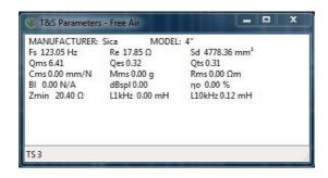
To get the complete set of Parameters load the Added Mass Impedance file and, again recall the CLIO Pocket Options, T&S Tab
