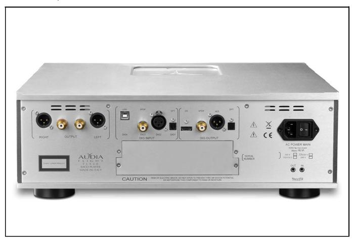
While we're on the subject of connectors, the FLS20 features inputs for USB-B audio, S/PDIF RCA coaxial, AES/EBU via XLR, and Toslink optical. Digital outputs include HDMI for I2S, S/PDIF RCA coaxial, AES/EBU via XLR, and Toslink optical. Analogue outputs cater to both balanced XLR and unbalanced RCA. An IEC socket coupled to the on/off switch and in/out 12V triggers round out the connectivity. At this point, I should mention the efficient rear panel layout and the first-class connector quality.
