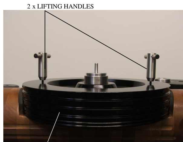
PHOTO 4 2 x LIFTING HANDLES LOWER PLATTER ONTO SPLINDLE
