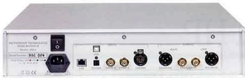
ABOVE: One Toslink optical, an AES/EBU and two coaxial digital inputs are joined by an asynchronous USB-Type B and an Ethernet port for network audio. Outputs include single-ended on RCAs and balanced via XLRs, at fixed level only
