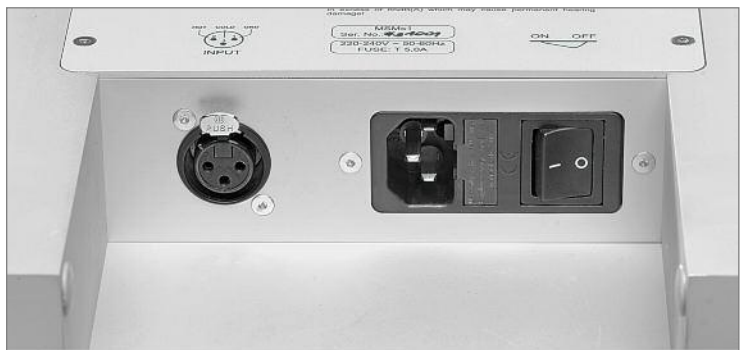
No frills: the connector panel consists of balanced input, power socket, and power switch
