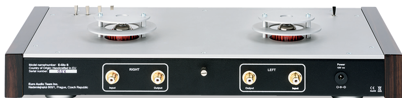
ABOVE: Simplicity itself – single gold-plated RCAs for connection to the tonearm leads and out to your choice of (pre) amplifier. Note \pm 18V DC PSU input socket
