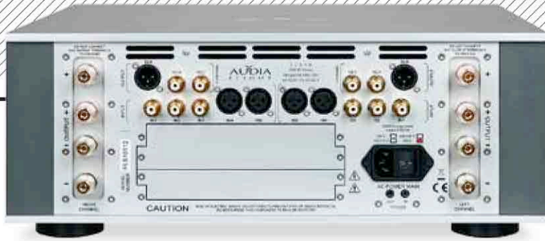
ABOVE: Five line-level inputs are offered, two on balanced XLRs and three on single-ended RCAs. Balanced and single-ended preamp outs are included alongside (fully floating) 4mm speaker outlets. Note access plates for optional DAC and phono boards
