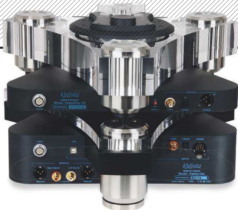
ABOVE: The DreamPlay CD transport [top] offers coaxial and optical S/PDIF outputs alongside AES/EBU while the Kalista DAC [bottom] has matching digital inputs plus USB-B. The balanced (XLR) analogue outputs are transformer-coupled
