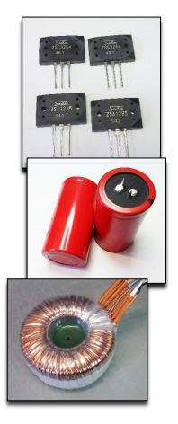
2 pairs per channel of high-quality C<sub>3264</sub> / A1295 ensure high output current in any load condition and high reliability
