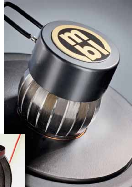
The Radialstrahler for the middle and high frequency ranges consist of narrow, stiff carbon lamellas coated with special lacquer which are distorted by the oscillation coils.
