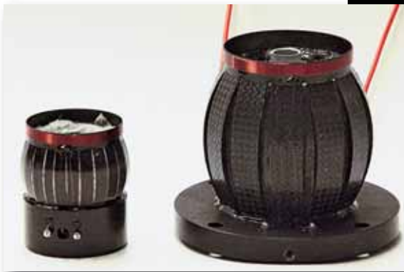
The Radialstrahler for the middle and high frequency ranges consist of narrow, stiff carbon lamellas coated with special lacquer which are distorted by the oscillation coils.
