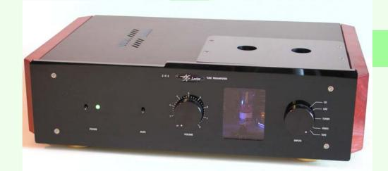
Stereo tube line preamplifier with two double triode in class A configuration.
