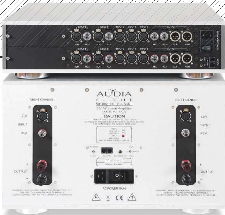
ABOVE: The preamp [top] offers five line inputs (two on XLR and RCA), two balanced outputs, one single-ended and one tape out. The power amp [bottom] has balanced (XLR) and single-ended (RCA) inputs with fully floating (ungrounded) 4mm speaker outputs
