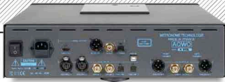
ABOVE: Two Toslink optical, two AES/EBU and two coaxial digital inputs are joined by an asynchronous USB-Type B. Outputs include single-ended on RCAs and balanced via XLRs, plus digital on Toslink, coaxial, AES/EBU and DSD as PS on an HDMI socket
