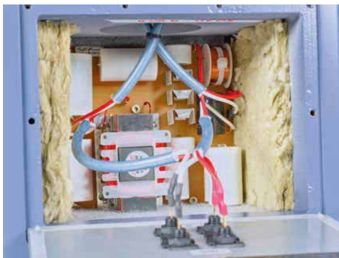
As was to be expected, the loudspeaker crossover is of very high quality and neatly assembled.
