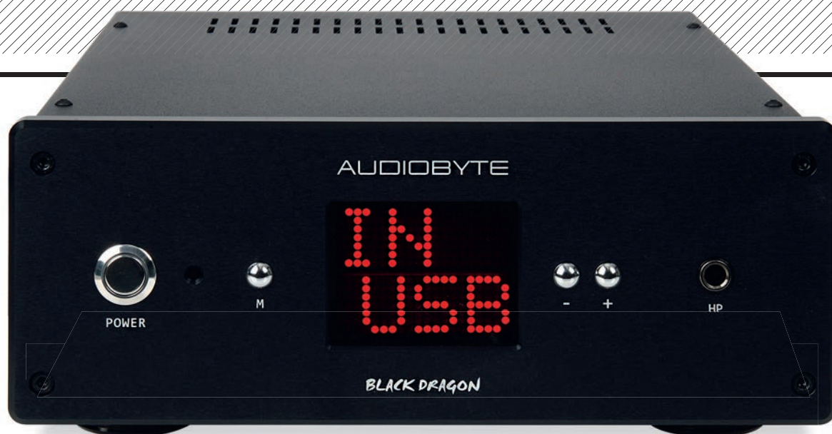
LEFT: Minimalist front panel includes an IR sensor and 6.35mm headphone socket. Menu 'M' and \pm buttons offer volume and input selection. Retro red dot-matrix screen is highly legible
