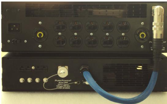
After initial start up it is acceptable to keep the APS on at all times. In standby the unit will only consume 10 watts. Battery charging will continue with the unit turned Off so long as it is plugged in to an AC supply and the input circuit breaker is switched on.
