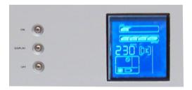
During startup the APS will operate in Bypass mode for a few seconds, then turn on its output - indicated by the LCD display icon "Online". When the "Online" indicator is illuminated, power is being supplied to the PurePower output receptacles. The PurePower APS is now ready to supply power to your system. Turn on the components, ensuring that the total load does not exceed the capacity of the PurePower 1500. The load usage will be indicated by the bar graph at the top of the display.
