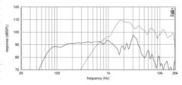
FREQUENCY RESPONSE MADE IN 25 LT. ENCLOSURE TUNED AT 65 Hz IN FREE FIELD (4 $\pi$ ) ENVIRONMENT. ENCLOSURE CLOSES THE REAR OF THE DRIVER, THE THIN LINE REPRESENTS HIGH FREQUENCY
