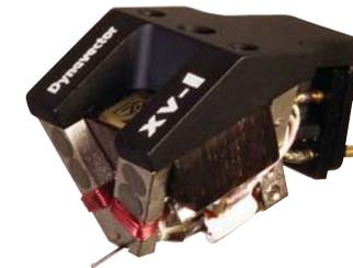
The XV-1s has a unique magnetic circuit. It comprises 8 small alnico magnets. The magnetic path is then divided into two. In the magnetic gap, a specially designed magnetic flux equalizing piece is placed. On
