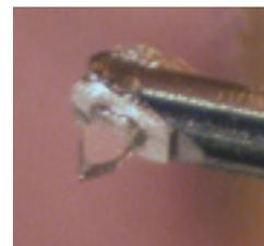
The clean diamond mount with alignment plate but with some excess adhesive above for this Dynavector
