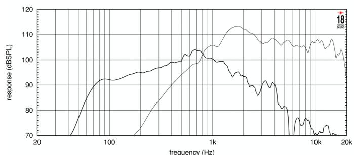
**FREQUENCY RESPONSE CURVE FOR THE SPEAKER LOADED IN A 50 LT ENCLOSURE TUNED 60 HZ IN FREE FIELD (4PI) ENVIRONMENT. ENCLOSURE CLOSES THE REAR OF THE DRIVER. THIN LINE REPRESENTS HIGH FREQUENCY RESPONSE**
