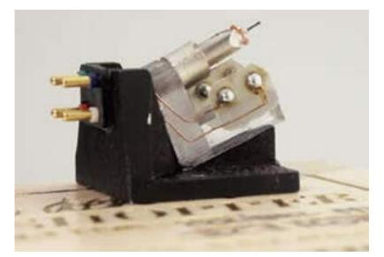
Notice the short cantilever made of boron and the microscopic needle. You can also see the little coils that just miss the vinyl. It is necessary to adjust the VTA about 4 millimeters higher than normal.
