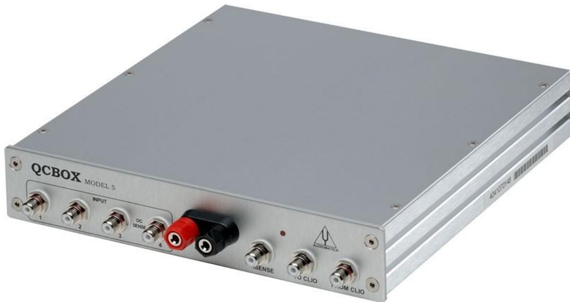
The QCBOX Model 5 switching and testing box is of invaluable help in everyday laboratory use and when configuring an automatic or manual quality control setup.
