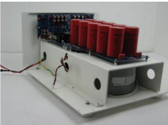
This stage is completely discrete components, is seen similar to an OpAmp and allows sonic superiority to amplify the current signal. The HDCA circuit has a bandwidth of 1Mhz, a distortion close to 0.00001%, linearity within 0.1db between 1hz and 250.000hz always guaranteeing a perfect interfacing with any source.
